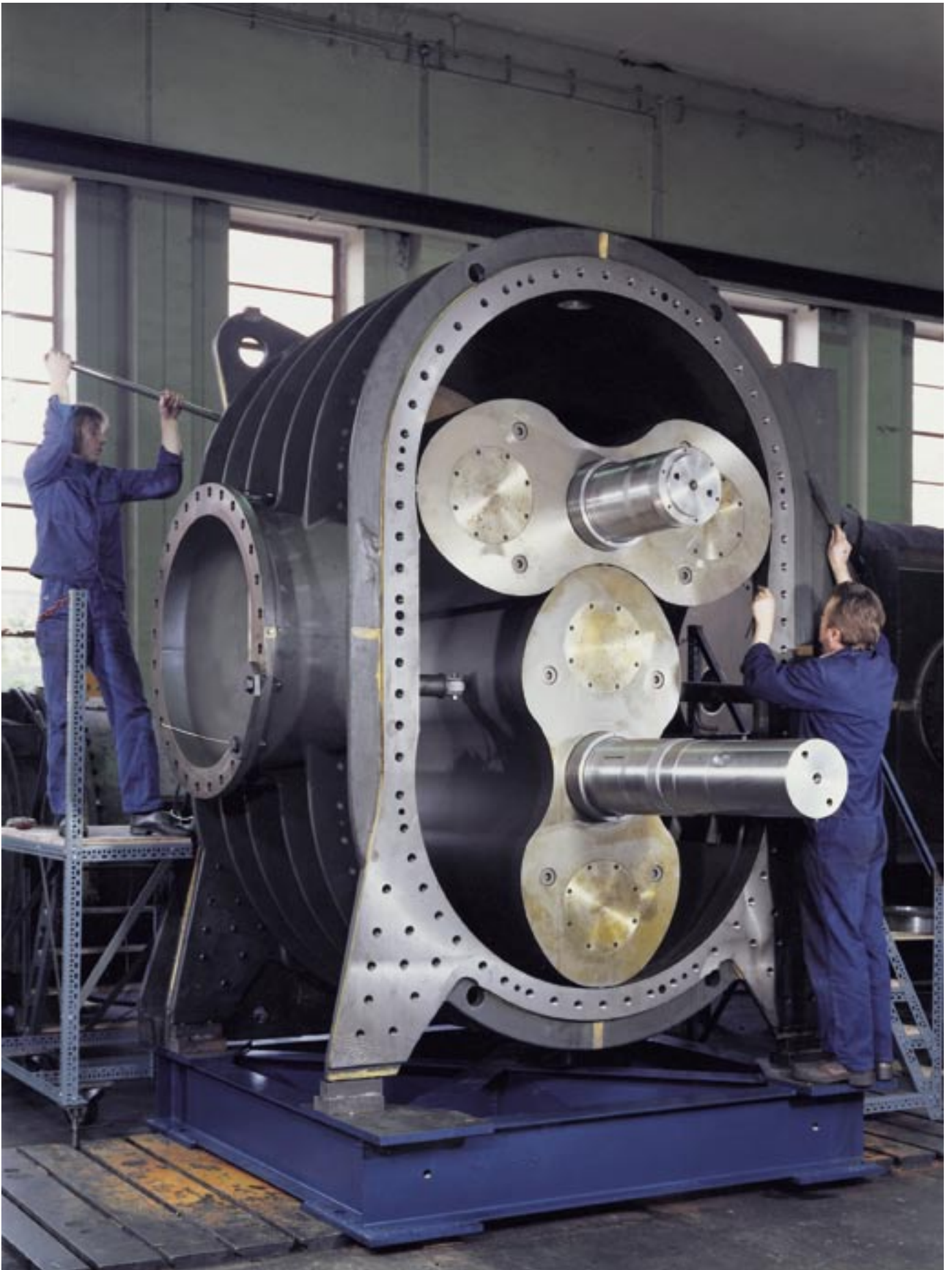
The largest Aerzen Positive Displacement Blower for the conveying of 100.000 m 3 /h gas, pressure difference 860 mbar, in a steel cooling plant. Length 3750 mm, width 2400 mm, height 3000 mm, engine output 3300 kW, weight 28 t.
