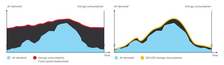
In almost every production environment, air demand fluctuates depending on different factors such as the time of the day, week or even month. Extensive measurements and studies of compressed air demand profiles show that many compressors have substantial variations in air demand. Only 8% of all installations have a more stable air demand.
