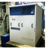
One of the world's leading suppliers of cement and aggregates was impressed by the low speeds of the Robox Screw, and thanks to the new Robuschi package has solved its breakdown problems with screw machines. Before installing the Robox Screw, dust in the atmosphere would enter the previous screw unit, which, when combined with the high-speed operation of the compressor (causing high temperatures on the shaft sealing) would result in damages to the machine.
