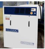
One of the European leaders in the production of disposable plastic tableware and food containers, collaborating with leading international distribution chains too, replaced old vacuum technology with the Robox Screw in vacuum operation. The unit is working at 300 mbar(a) with a consistent energy savings (up to 30kW/h comparing to the previous technology).
